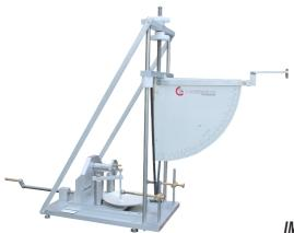
MODEL . . . . . IMPACT TEST ASTM FOR **TABLEWARE**
